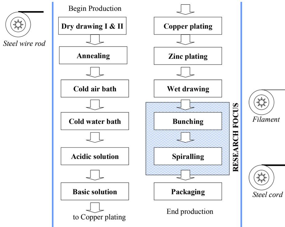
Figure 2. Production Processes in Steel Cord Manufacturing
