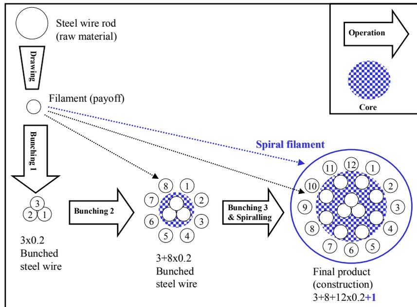
Figure 3. Cross-section of  $3+8+12 \times 0.2+1$  Construction at Successive Bunching Operations
