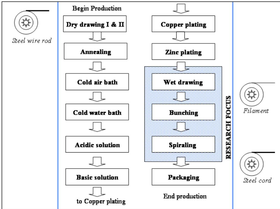
Figure 2. Production processes in steel cord manufacturing
