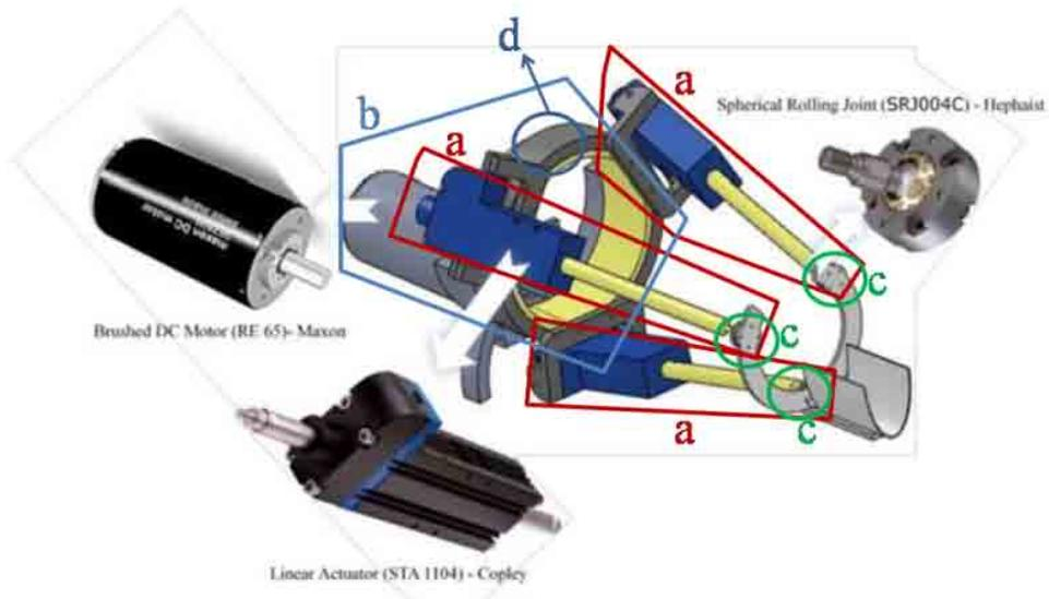
**FIGURE 3.** SECOND VERSION OF THE ASISTON-WRIST ROBOT [37]
