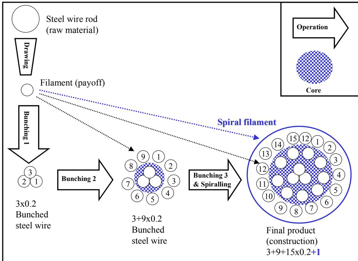
Figure 3. Production Processes in Steel Cord Manufacturing
